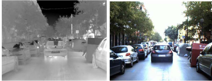
Figure 2.2: Thermal (left) and visible-spectrum (right) image of the same scene. Source: Mouats et al. [25].
