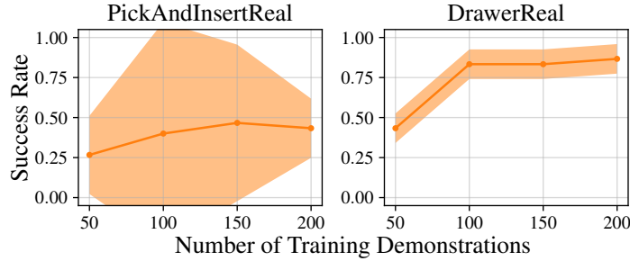
Figure 3.7: Performance results for the other real environments in which we only tested multiview policies. The shaded region shows the two-sigma bounds across three policy seeds.
