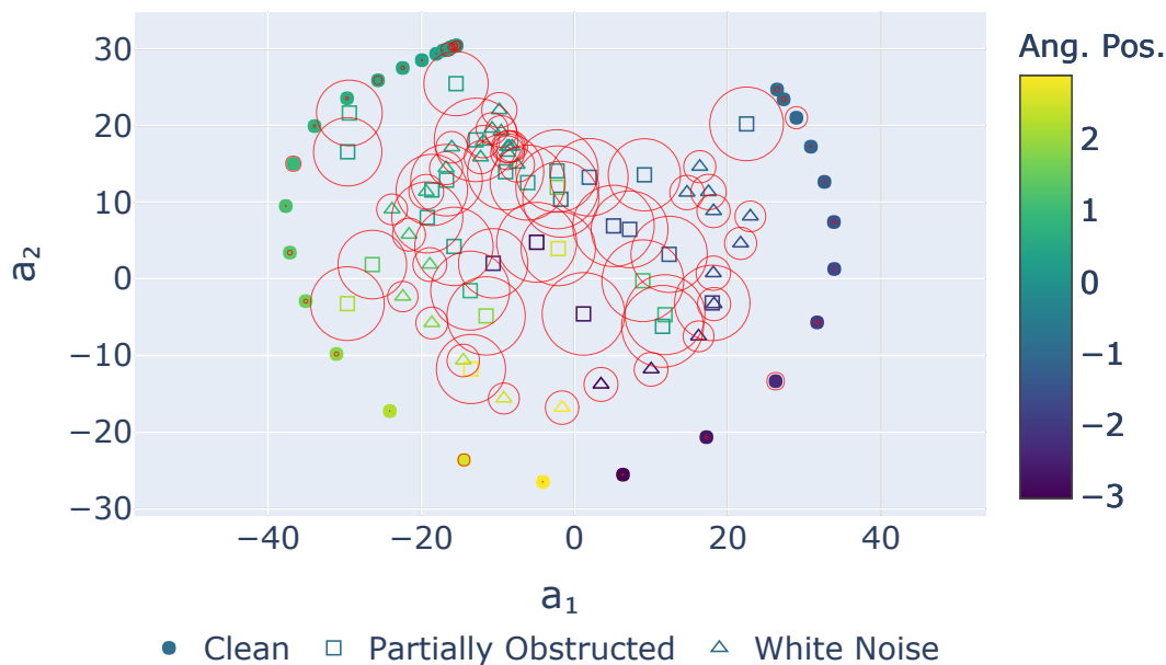
Figure 3.4: The extracted latent measurements for the pendulum task, \mathbf{a}_k \in \mathbb{R}^2 , from clean images (filled circles) and corrupted images (hollow squares and triangles) with their respective covariances (in red). Note that the covariances of the clean measurements are small and more difficult to visually distinguish.
