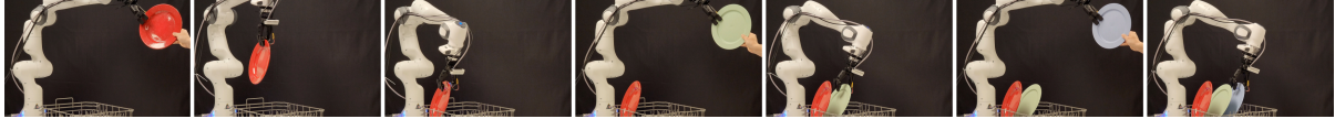
(a) dish rack placement task, which consists of placing multiple plates of varying physical properties in evenly spaced slots.
