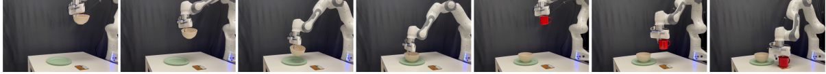
(b) Table placement task, which consists of placing a bowl on a plate and a cup on a coaster.
