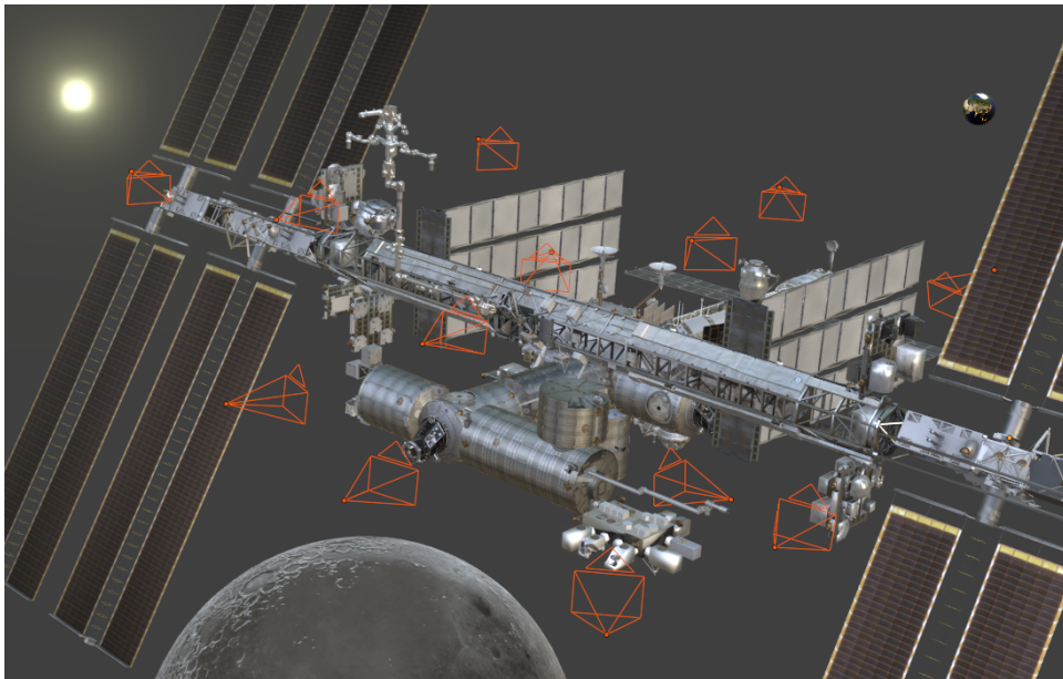
Figure 4.2: Blender model with example camera positions (highlighted in orange) around station.
