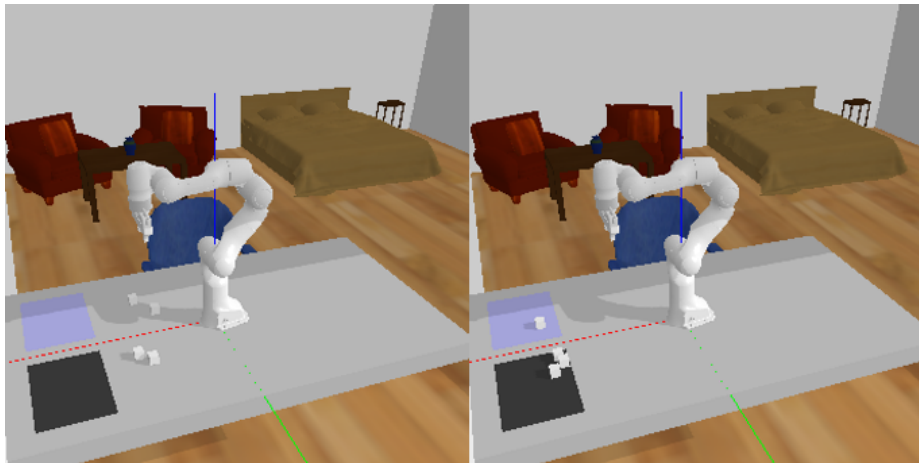
Figure 5.3: A graphical view of sorting experiment: Left: The initial state, where three cubes sparsely sit on the table. Right: The goal state, where the cubes are clustered into two piles.
