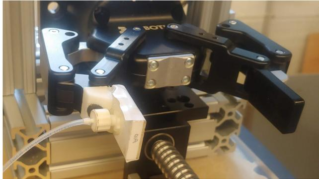
(c) Gripper with one of its original ('stock') fingerpads replaced with an adaptive fingerpad, viewed from the front. An air supply tube is connected at the back of the adaptive fingerpad.
