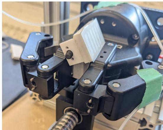
(b) Front side and base of an adaptive fingerpad. The active regions of the fingerpad surface are visible under the (translucent) top layer.
