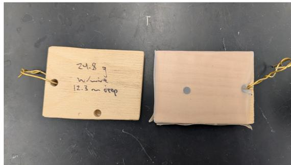
Figure 7.8: Target blocks for shear tests. Left: bare plywood. Right: wrapped with PTFE tape.
