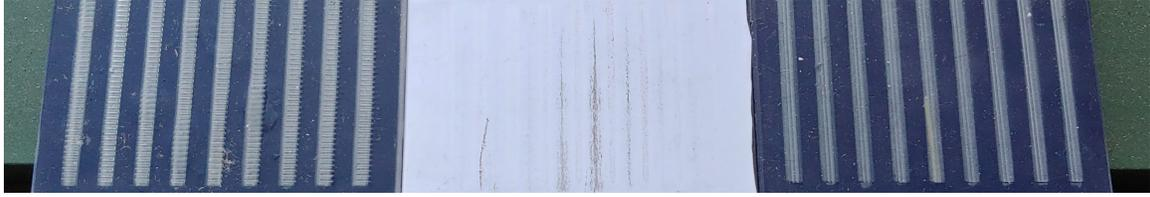
Figure 6.3: The three adaptive surface devices used in flat device testing, pictured after all tests had been completed. The PVC device (centre) shows some visible wear as dark streaks along the active region edges, and the printed device with the short widthwise ridge features (left) shows some defects from excess resin deposition during printing that are not visible on the printed device with the long lengthwise ridge features (right).
