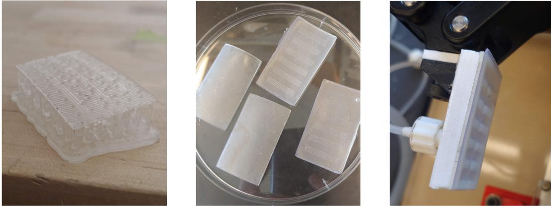
(a) Printed surface, with supports. (b) Printed surfaces, no supports. (c) Fingerpad with printed surface.
