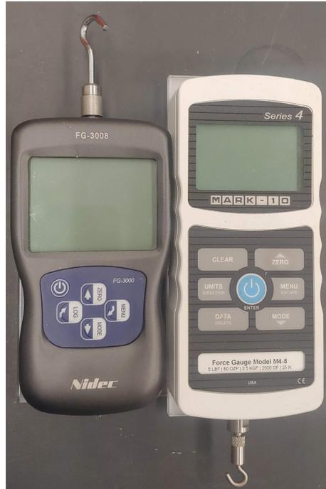
Figure 5.5: The two force gauges used in shear testing. The Mark-10 M4-5 gauge (top) has a capacity of 25 N with a resolution of 0.01 N. The Shimpo FG-3008 gauge (bottom) has a capacity of 500 N with a resolution of 0.1 N.
