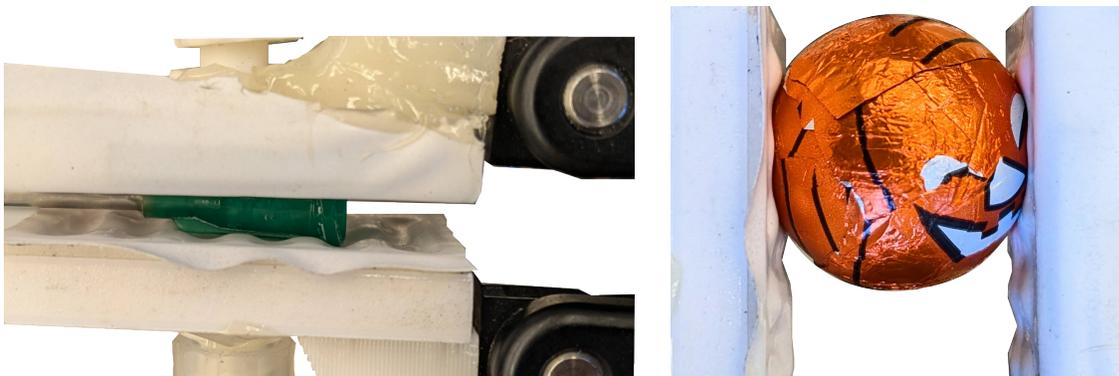
(a) Interlocking between flange of cannula fitting (green) and deflated fingerpads.
