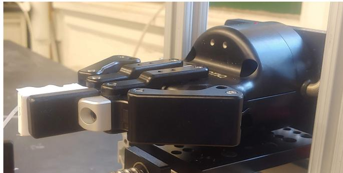
Figure 4.13: Gripper with one adaptive fingerpad and one stock fingerpad. Fingerpad edges are misaligned because of uneven adhesive application between the adaptive fingerpad and its mount.
