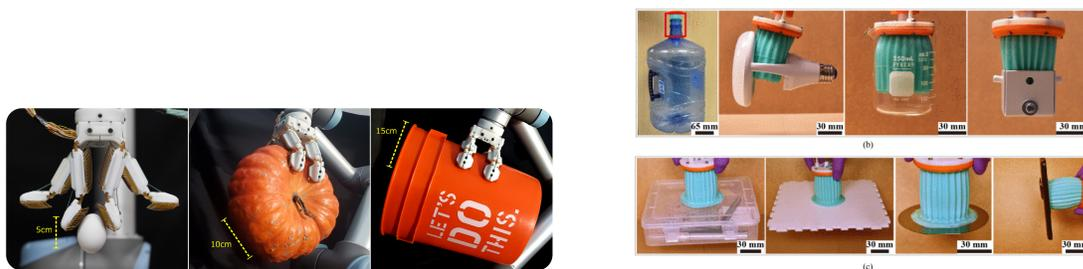
(a) Multifingered gripper demonstrating different types of impactive grasps. Figure and caption adapted from Ruotolo et al. [11] with permission from AAAS.
