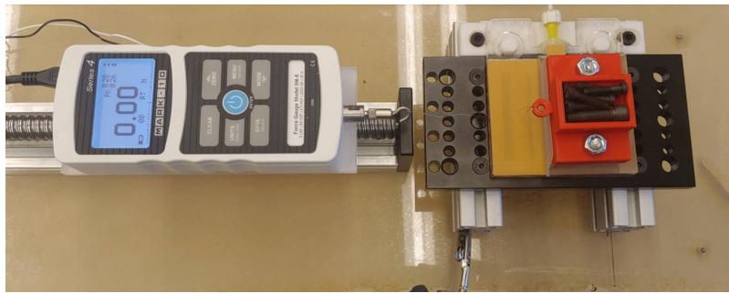
Figure A.2: Baseline flat device test setup. The device is fixed to the test platform, which acts as a lower constraint. The sled rests freely atop the device and is pulled across the device by the gauge.
