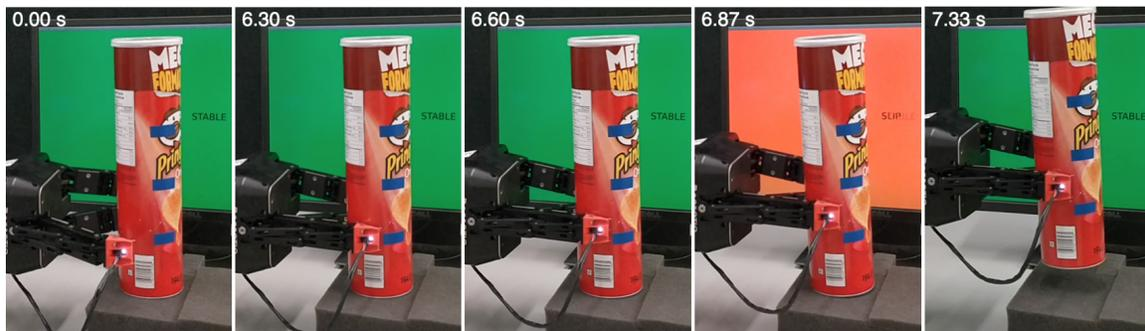
Figure 5.6: Object-lift test with the cardboard can, showcasing a successful trial. The time stamps were extracted from the video and may not be accurate.
