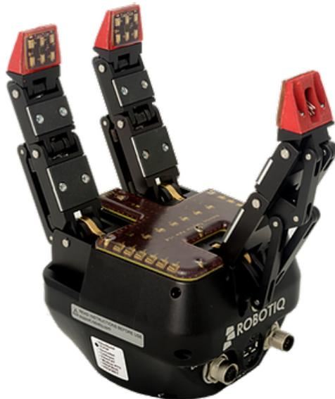
Figure 4.1: Robotiq three-finger adaptive gripper, retrofitted with the TakkTile sensor kit (image from [54]). The single finger on the right is referred to as the ‘thumb’ of the gripper.
