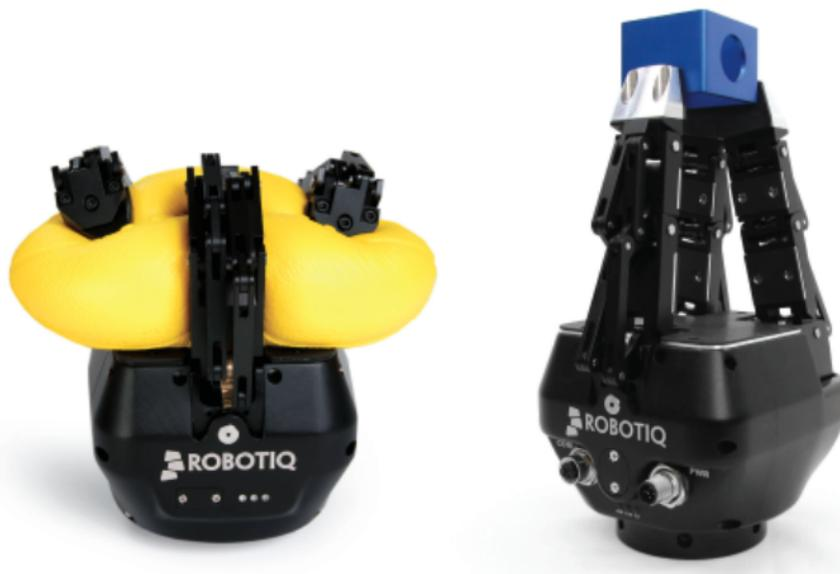
Figure 4.2: Power grasps of the Robotiq gripper (sourced from [54]). An object is held firmly between the fingers and the palm for the sphere grasp (left), whereas for the pinch grasp (right) the object is held solely by the fingertips while making no contact with the palm region.
