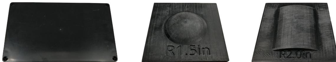
Figure 4.5: Surfaces used for slip data acquisition; from left to right the images show a planar box lid, a spherical plastic surface (radius 1.5 in), and a cylindrical plastic surface (radius 2 in).
