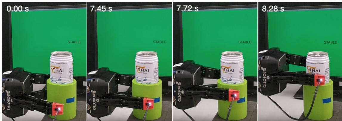
Figure 5.7: Object-lift test with the foam sleeve, showcasing a failure trial. The time stamps were extracted from the video and may not be accurate.
