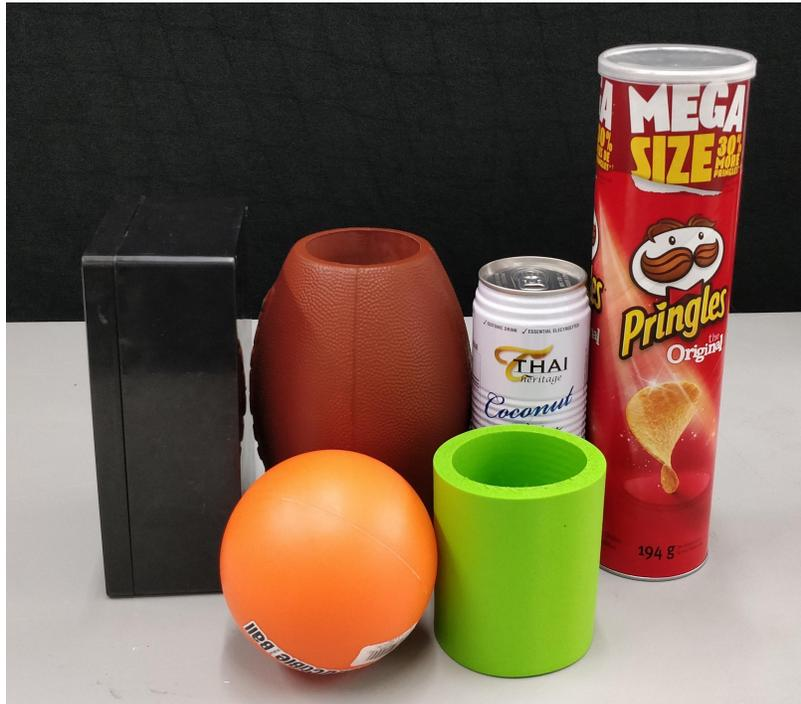
Figure 5.2: Test objects used for robot experiments. From left to right, the objects are: *plastic box* , *plastic ball* , *football sleeve* , *foam sleeve* , *metal can* , and *cardboard can* .
