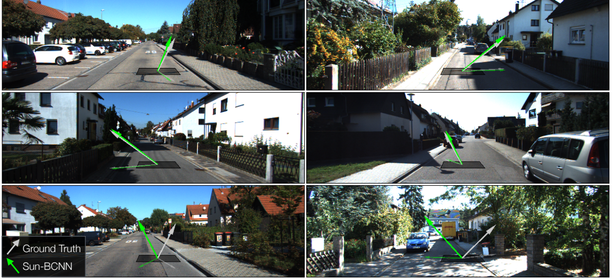
Figure 3.12: Visualization of Sun-BCNN predictions and associated ground truth sun directions on KITTI sequence 05. Top two rows : Sun-BCNN produces accurate predictions in a variety of azimuth values. Bottom row : Poor results occur rarely due to shadow ambiguities.
