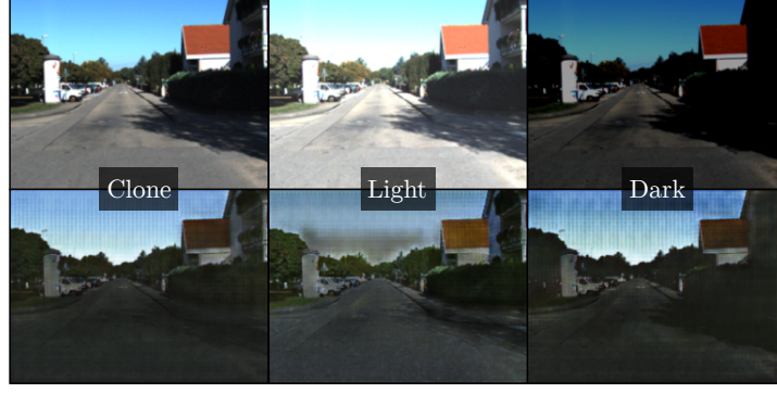
Figure 4.6: Top row : Sample images from the KITTI/05 sequence (Geiger et al., 2013) from the same pose under different affine brightness transformations. Bottom row : The same images with a learned transformation that attempts to re-illuminate each image under the VKITTI “Overcast” condition.
