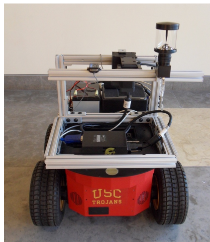
Fig. 2. Pioneer 2-AT mobile robot, equipped for calibration experiments. The NetVision 360 omnidirectional camera lens is visible in the upper right.
